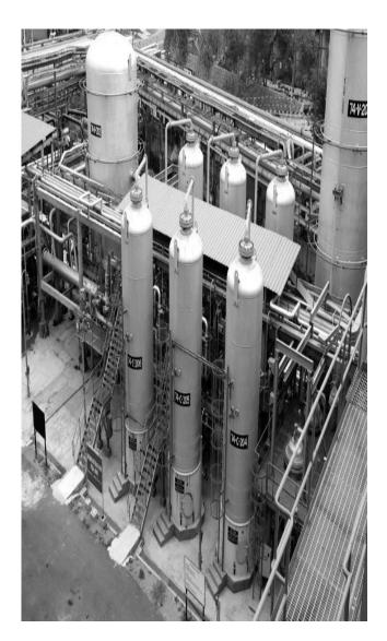
H2 PSA Technology is being offered by HPGRDC along with its Korean partner for  $H_2$  purification in process industries.
